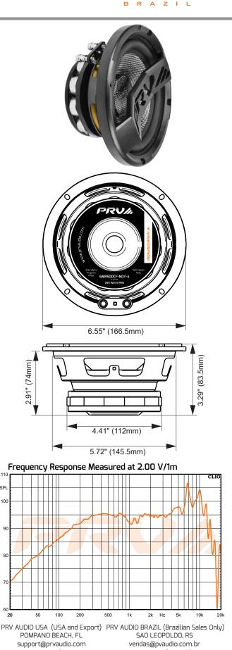
\*\*Xmax=(Voice coil winding depth-Magnetic Gap depth)/2+ Mgnetic Gap Depth/4 \*\*\* T-S parameters measured after 2 hours at 1/2 Rated power, pink noise preconditioning test dBSPI 100
